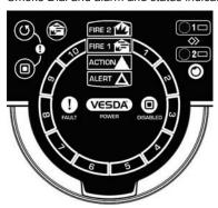
When the field service access door is open, the user has access to the RESET \( \mathcal{O} \) DISABLE , Fire Test , AutoLearn and Instant Fault Finder functions. When the Instant Fault Finder function is activated, the Smoke Dial converts to a fault indicator, with the dial segment numbers corresponding to the faults listed below.
